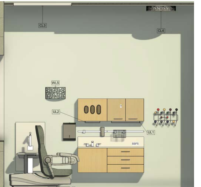
EXAM ROOM NORTH ELEVATION
